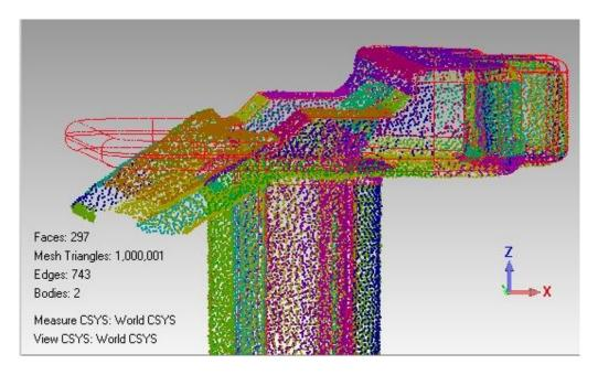
The correspondence algorithm applies an intelligent search based on the normal approximation of the test data. The algorithm utilizes topological and geometric classification techniques that were first developed in the functional decomposition approach [13,16].
