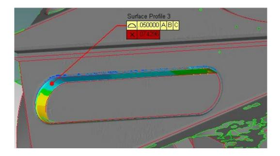
Summarily the usage of the correspondence mapping enables the total automation of the inspection process. Once we have the reference CAD model together with inspection directives (possibly in the form of PMI information) and the suitable non-contact (scanned) measured data of the part is available, then the full inspection report can be obtained in a fully automatic way.
