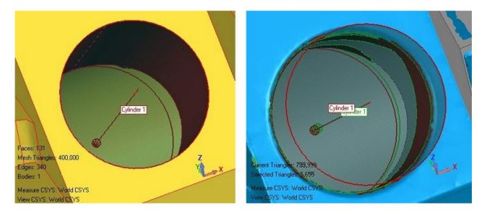
When activating this procedure the subset of the measured data is retrieved that corresponds to the reference feature and a fitting algorithm is performed to create a feature attached to the test object.
